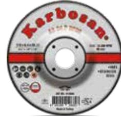
Suitable for grinding process of high alloy steels, hardened steels, stainless steels and common steel cast materials. Featuring special aluminum oxide abrasive grains and a hard structure, the product is ideal for grinding stainless steel materials. The product does not contain iron (Fe) and sulfur (S).
