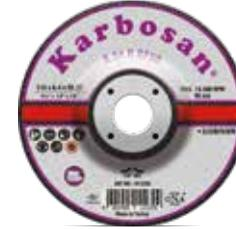
Suitable for grinding operations on aluminium, copper, brass and bronze materials. Featuring aluminum oxide abrasive grains and a hard structure, the product offers the advantage of convenient material removal without causing clogging.
