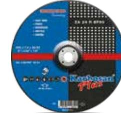
Suitable for grinding process of welding burrs and seams, high alloy steels, mild steels, stainless steels, spherical graphite cast iron, grey cast iron, common steel cast and sand finished surfaces. Featuring zirconia abrasive grains and a hard structure, the product offers the advantage of more aggressive material removal than standard products.
