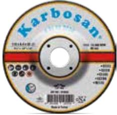
Suitable for grinding process of welding burrs and seams, all structural steels, high alloy steels, hardened steels, mild steels, stainless steels and common steel cast materials. Featuring aluminum oxide abrasive grains and a hard structure, the product offers long lifespan and advantage of quick cutting.
