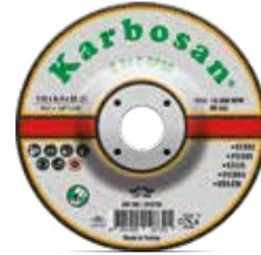
Suitable for grinding process of spherical graphite cast iron, grey cast iron, sand finished surfaces, copper, brass, marble, artificial and natural rocks. Featuring silicon carbide abrasive grains and a hard structure, the product offers long lifespan and advantage of convenient material removal.
